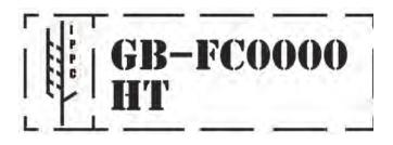
An example of a mark applied by stencilling; small gaps are permitted in the border, lettering and other elements.
