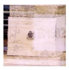
Example 3: Poorly Applied Wood Mark Where Registration Number is Absent or illegible
