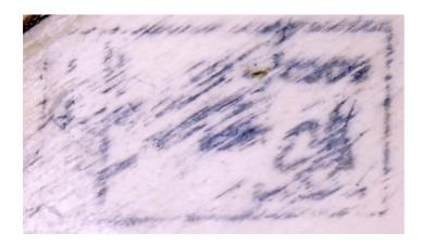
Example 2 : Faded Wood Mark ie not permanent on a Pallet Block
